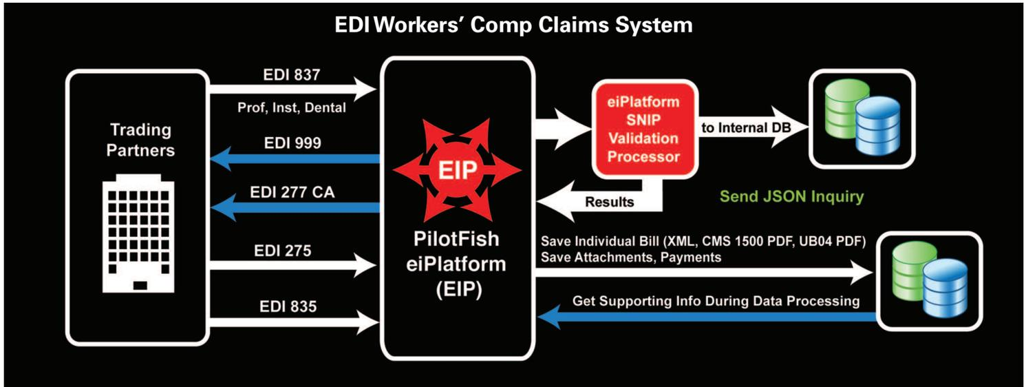
A batch workflow showing EDI 837 from a Trading Partner, ingested and traversing through the PilotFish SNIP Validation Processor then into an Internal DB which generates an EDI 999 and an EDI 277. The EDI 275 and EDI 835 from the Trading Partner's Source System is ingested by PilotFish as an individual bill with saved attachments and payments then transported as a JSON inquiry to the database which yields supporting info during data processing.
